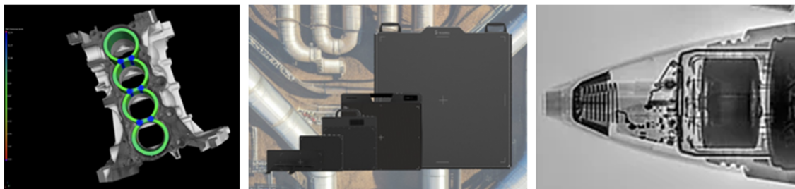
Figure 2. Examples of images generated from commercial x-ray radiographic systems and panels used to make those images. The left figure shows an image generated by VJTechnologies' Veda HE industrial system [76]. The center image shows a family of radiographic panels produced by Scanna [47], while the rightmost image is a radiograph obtained by a NOVO Systems detector [46].
